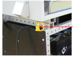
Quick Connect Propane Fitting on Fuel Cell
