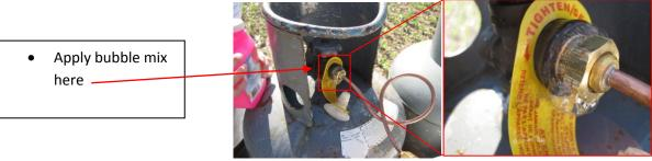
2. Attach the quick connect fitting on the manifold to the connector on the fuel cell.
