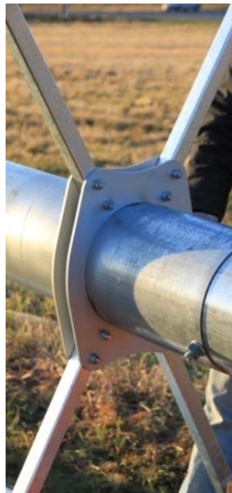
Picture 3-46: Jumper strut alignment
