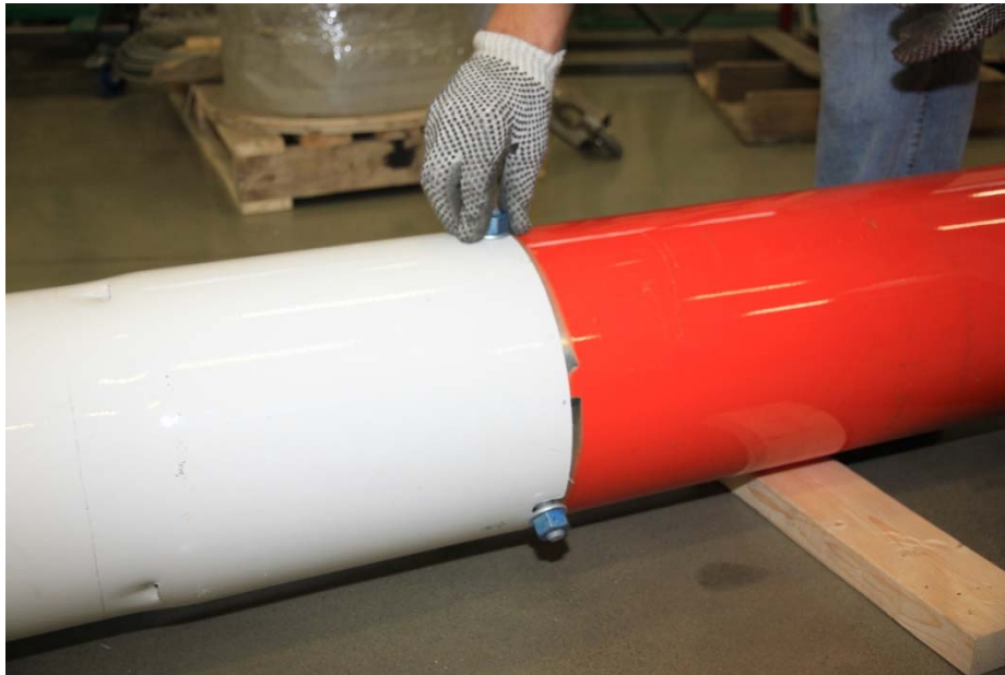
Picture 3-20: Nuts/bolts hand tightened
