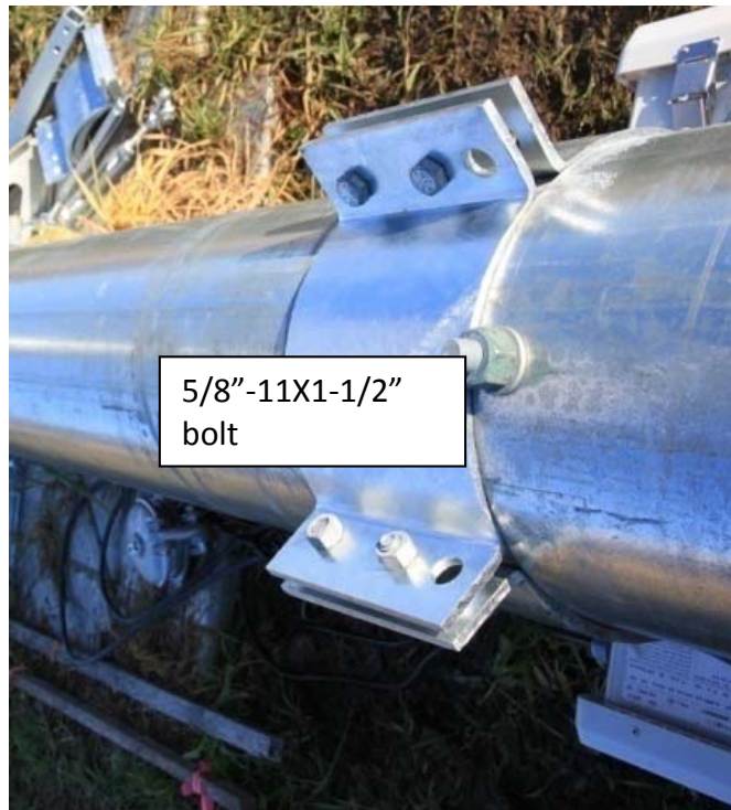
Picture 3-41: Ginpole jumper strut end-flange bolts
