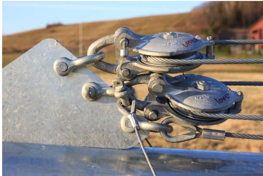
Picture 3-59: Correct block pulley assembly
