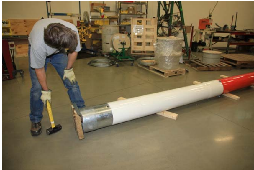
Picture 3-21: Seating the tubes with a mallet
