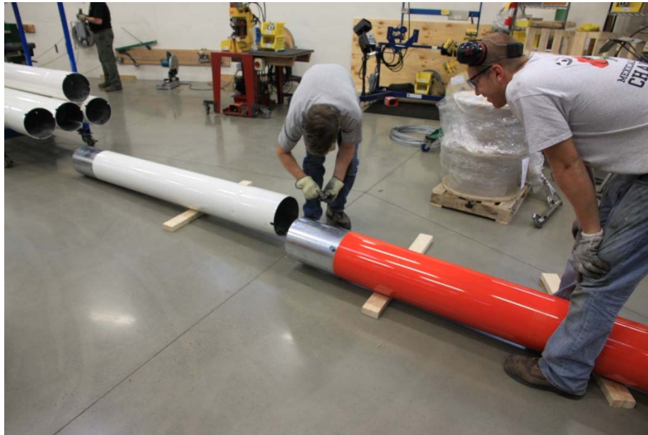
Picture 3-16: Attach tower bolt/nuts
