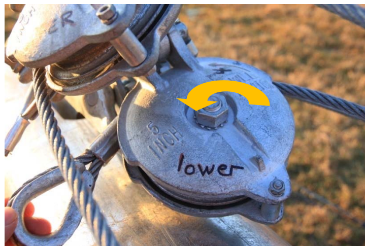
Picture 3-76: Reeving through pulley #4
