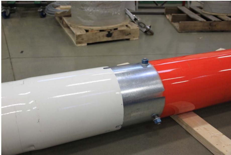
Picture 3-18: Sliding together tube sections
