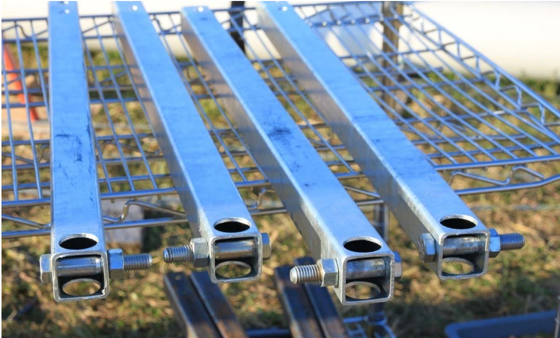
Picture 3-44: Install bolts/nuts onto jumper struts
