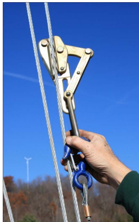
Picture 4-11: Using a Chicago grip
