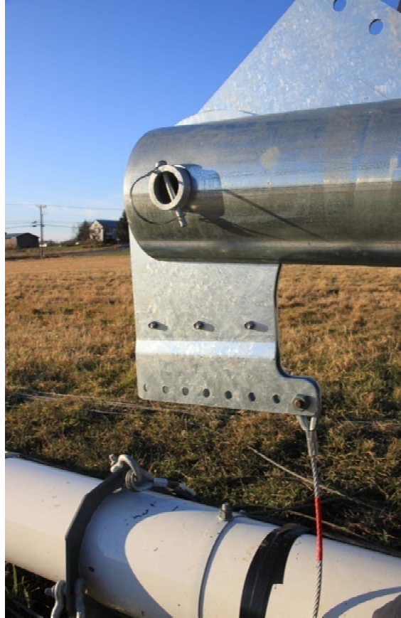
Picture 3-56: Lifter attachment to rocker plates
