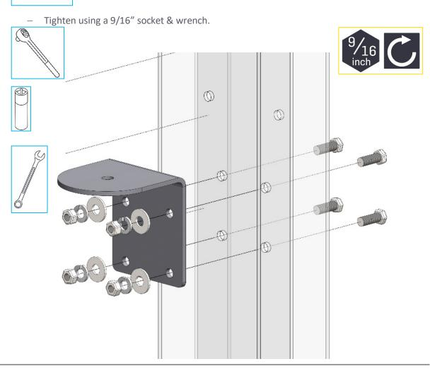
5 Torque the L-bracket mounting bolts to 15 ft-lbs (20.3 Nm).
