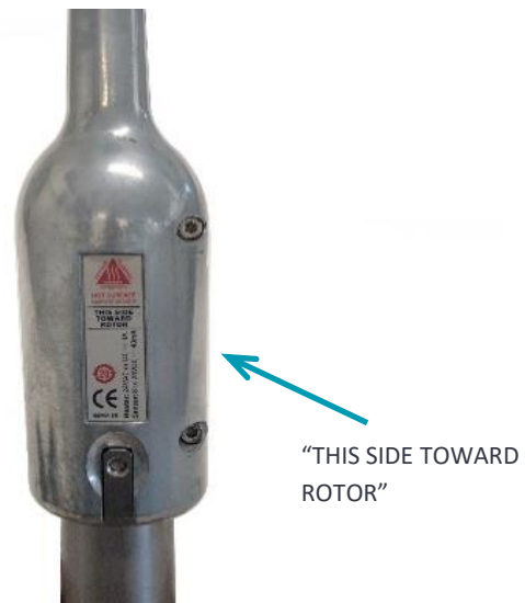
Slide sensor down over mast.
