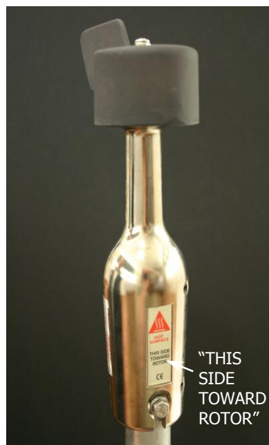
Slide sensor down over mast.
