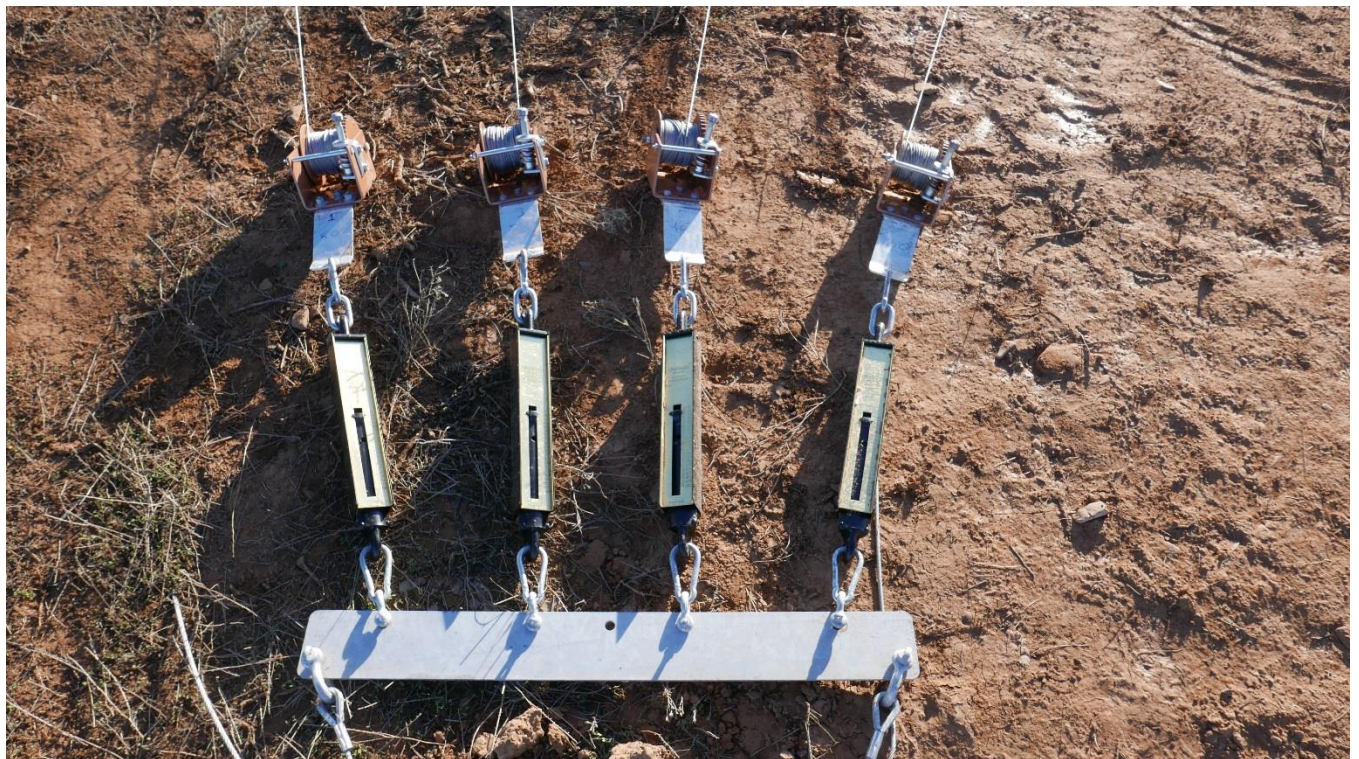
Picture E-8: Connecting the worm gear winch cables to the leader lines
