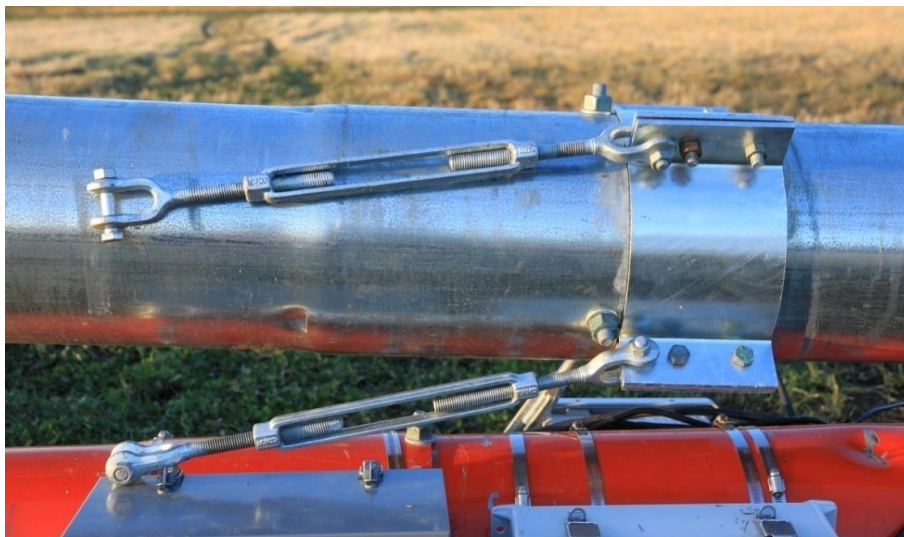
Picture 3-43: Turnbuckle assembly
