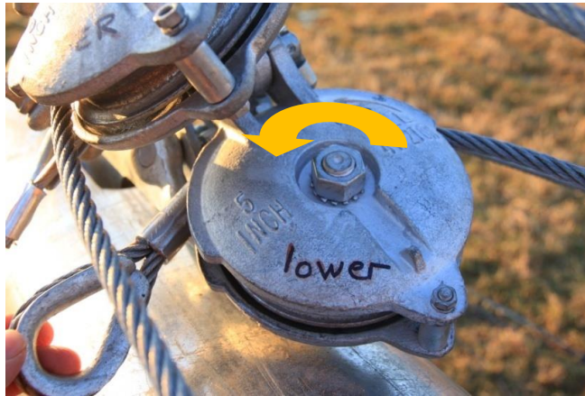
Picture 3-77: Reeving through pulley #4
