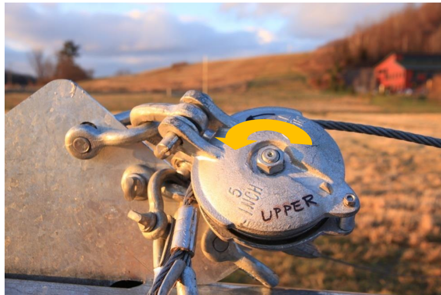
Picture 3-74: Reeving through pulley #2
