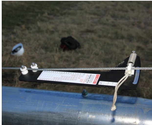
Picture 3- 81: Correct use of tension gauge
