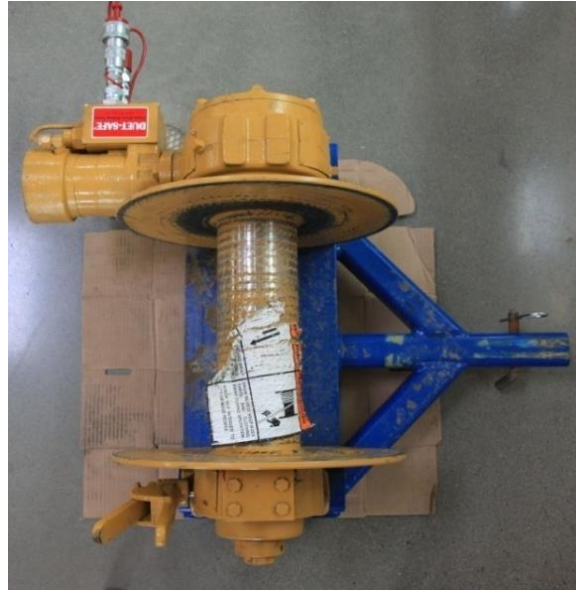
Picture 3-65: 80 Meter Bloom winch with mounting plate
