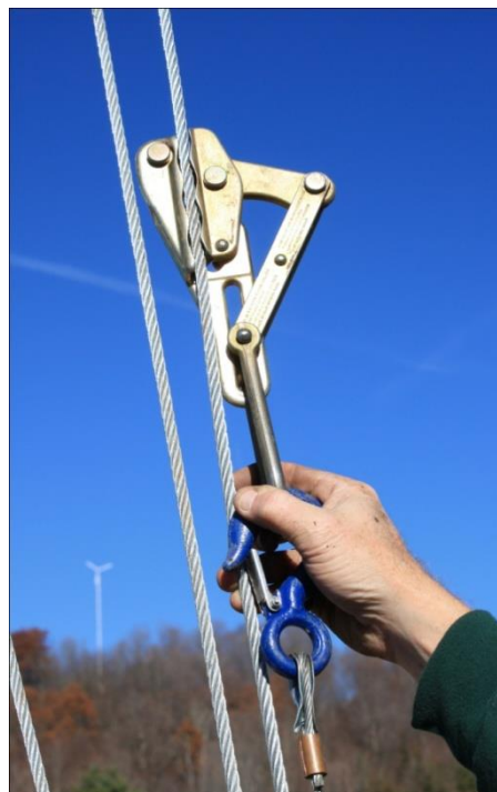
Picture 4-11: Using a Chicago grip
