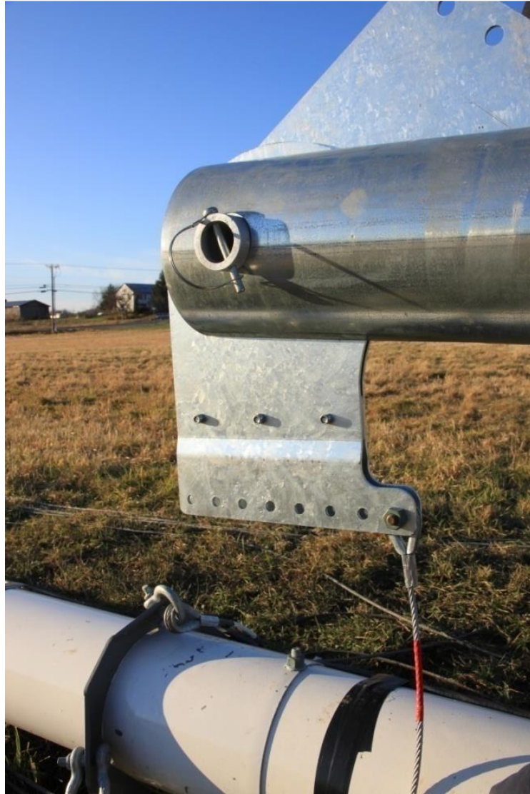
Picture 3-57: Lifter attachment to rocker plates
