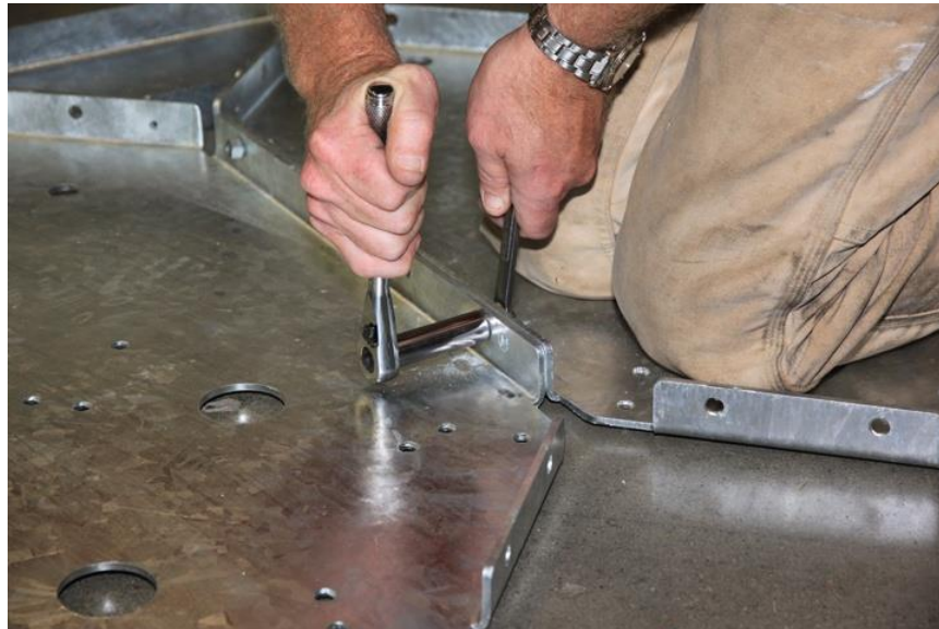
Picture 3-2: Baseplate Assembly
