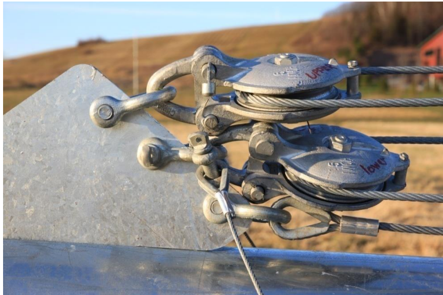
Picture 3-60: Correct block pulley assembly
