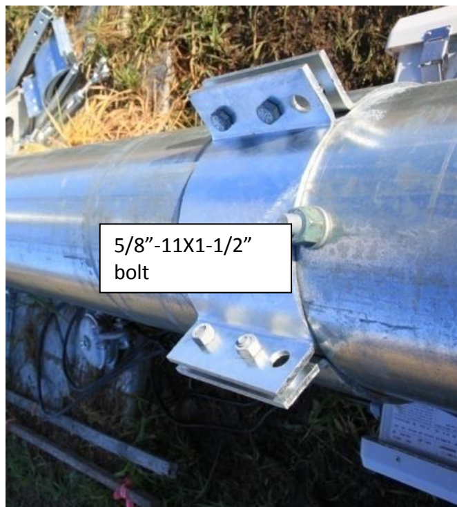
Picture 3-41: Ginpole jumper strut end-flange bolts
