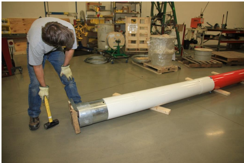
Picture 3-21: Seating the tubes with a mallet
