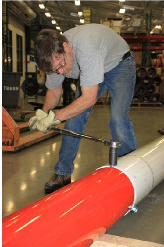
Picture 3-24: Torqueing the nuts
