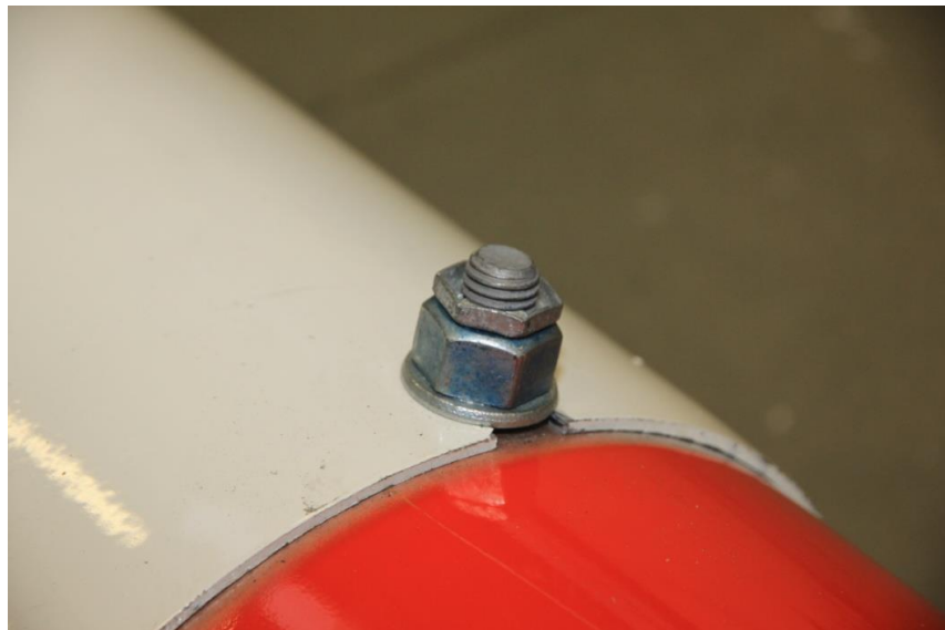
Picture 3-25: Tube joint fully torqued with palnut attached
