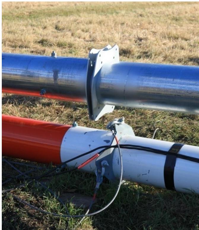
Picture 3-38: Jumper strut center ring plates
