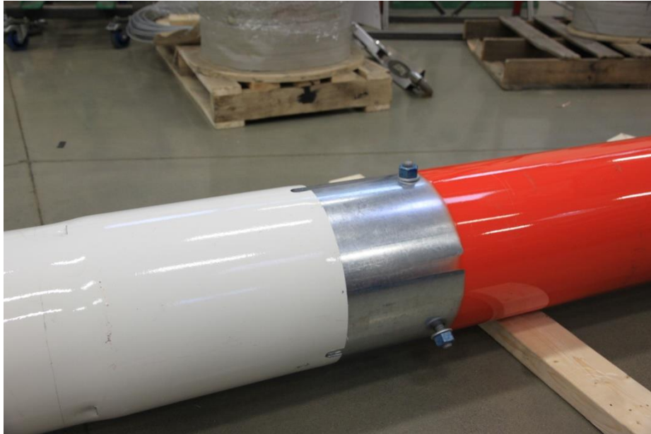
Picture 3-18: Sliding together tube sections
