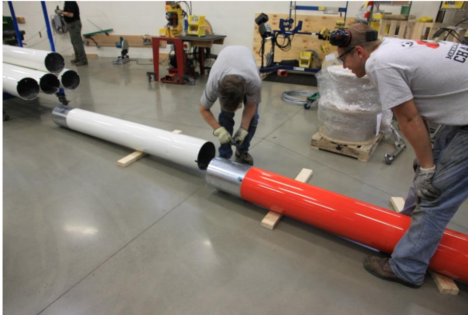
Picture 3-16: Attach tower bolt/nuts
