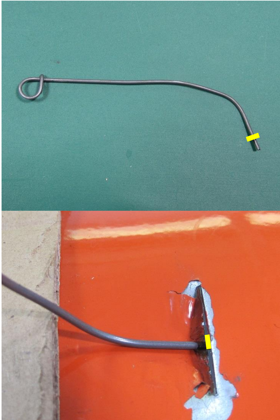
Picture 3-23: Example of tool that can be used to confirm tubes are mated together fully
