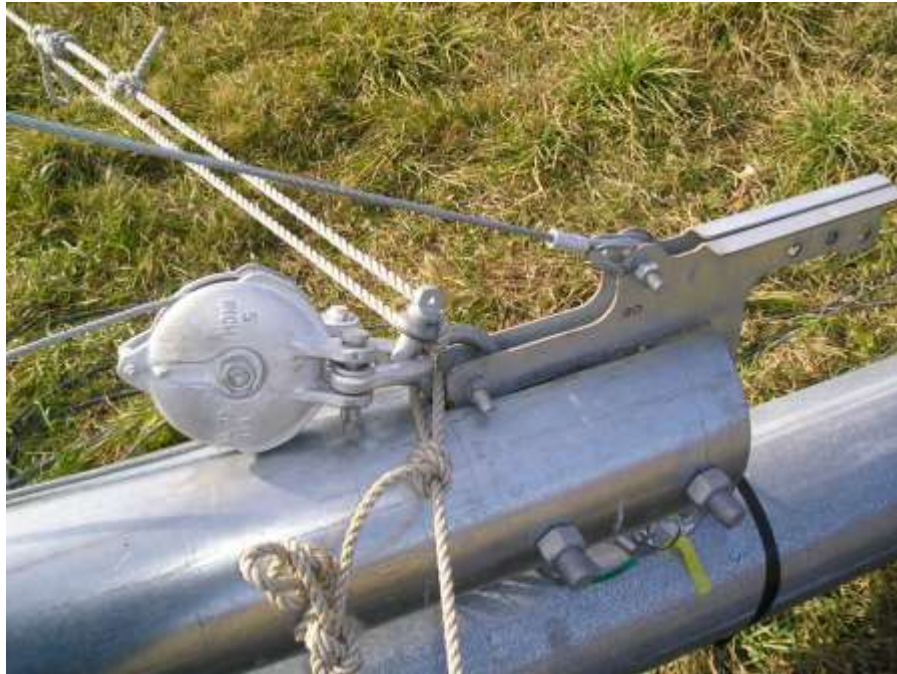
Picture 3-41: Winch cable attaches to top of ginpole
