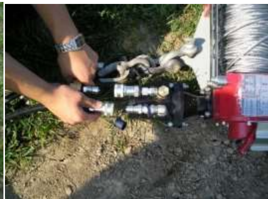
Picture 3-36: Hydraulic winch
