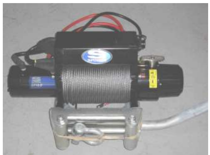
Picture 3-33: S900 electric winch assembly
