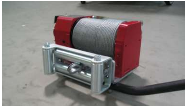
Picture 3-34: Hydraulic Winch assembly
