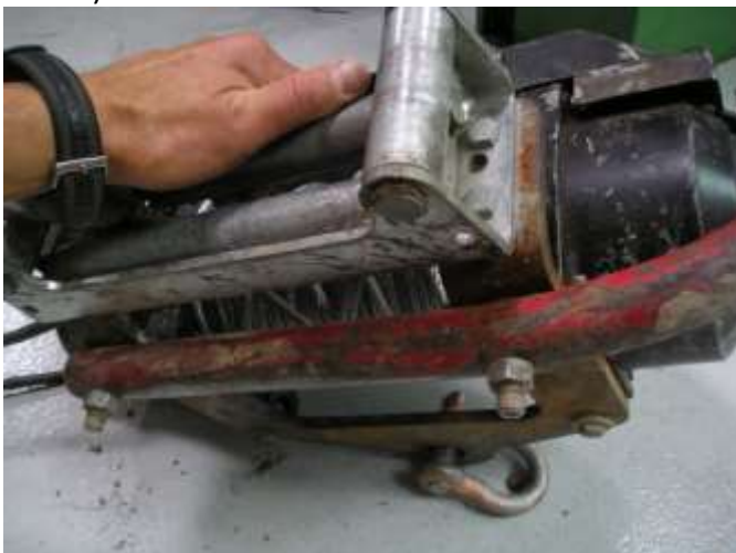
Picture 3-32: Old winch control bar attachment
