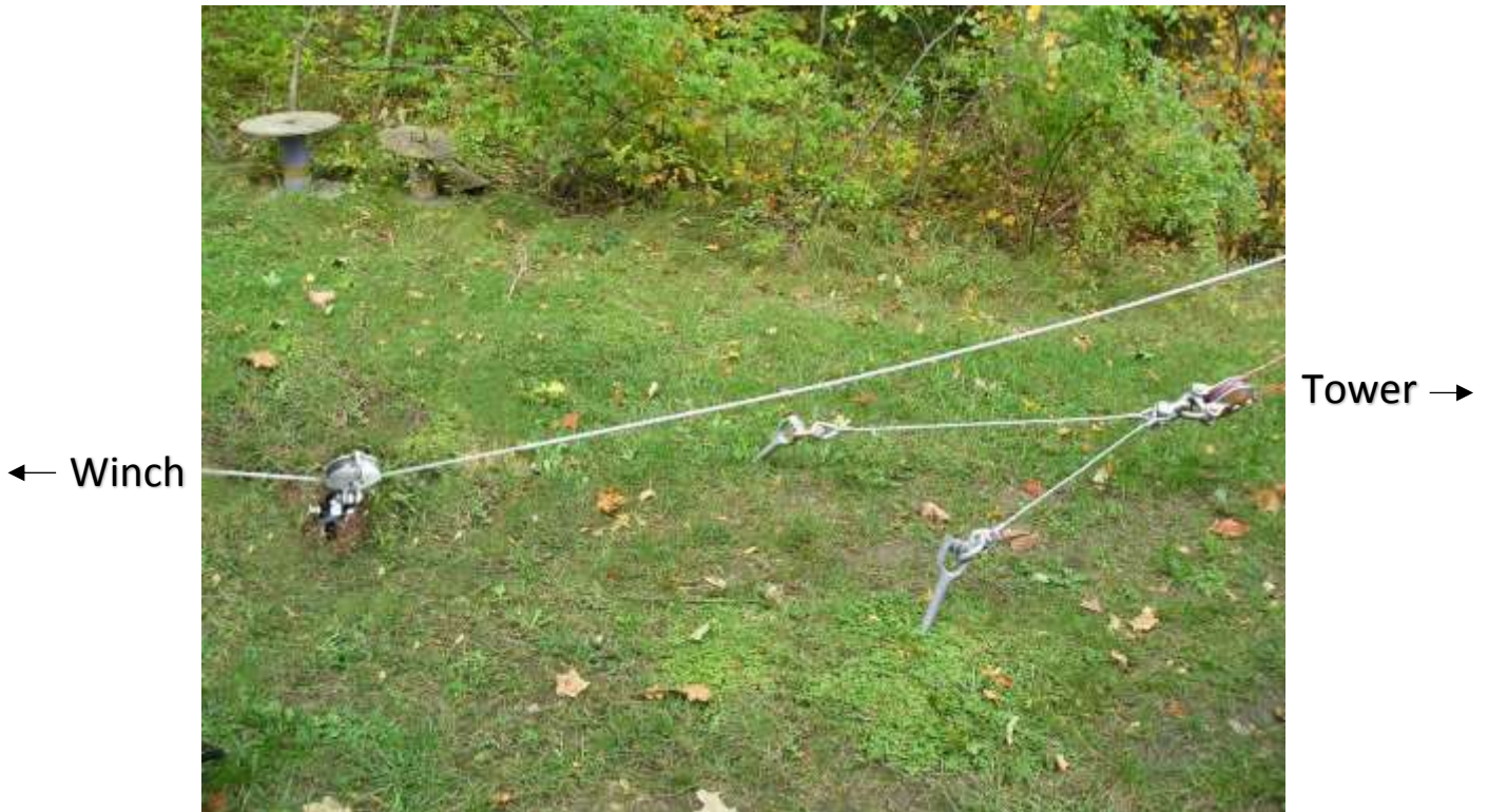
Picture S-8: Bridle cable assembly with extra block pulley for use with 80m winch
