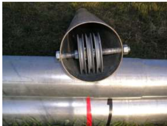
Picture 3-30: Ginpole top tube sheave attachment
