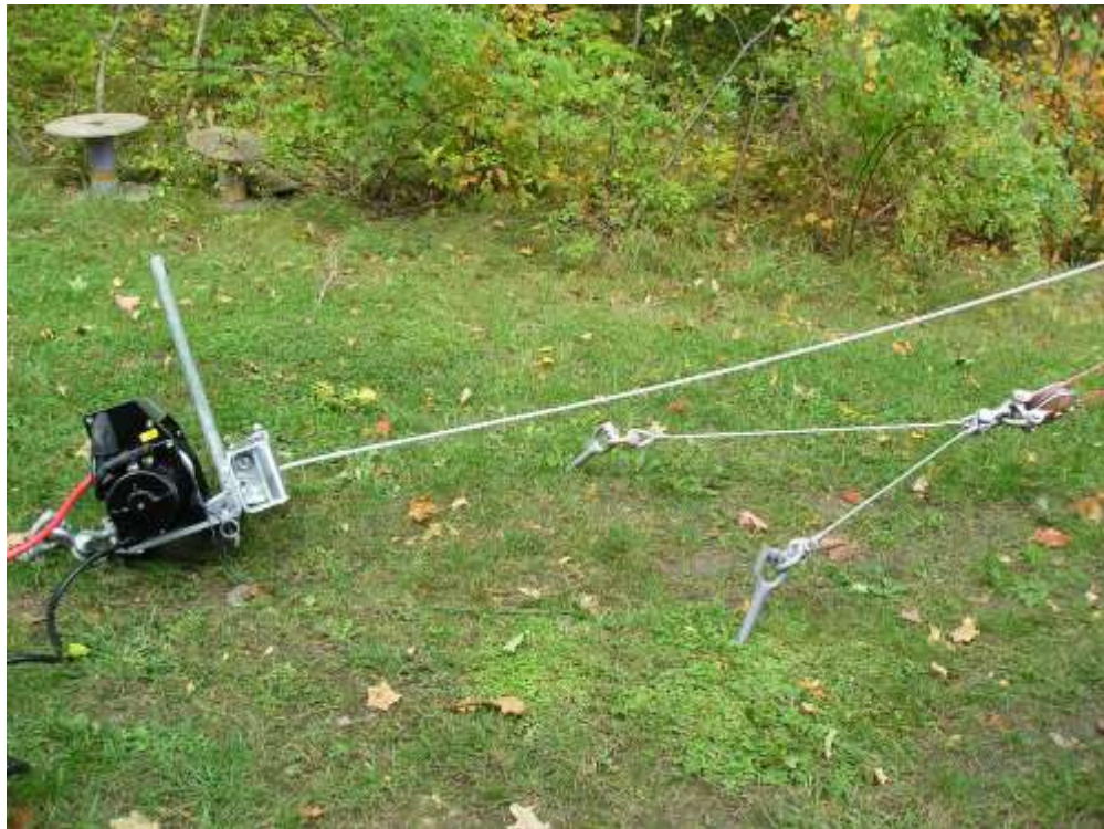
Picture 3-38: Winch & Bridle Assembly set-up
