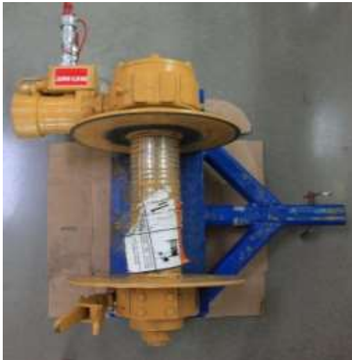
Picture S-2: 80 Meter Bloom winch with mounting plate
